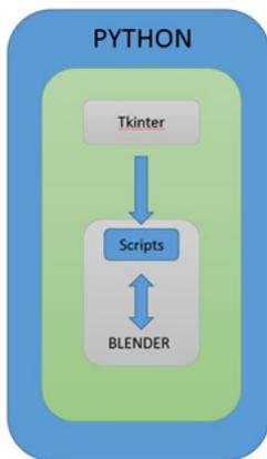
**Fig. 1.** Schematic Diagram of the graphic simulator. Tkinter GUI selects which script to run and the chosen script is executed for modification of the objects or animation.
