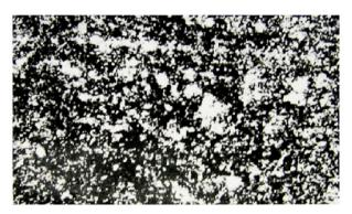
Figure 3. Micrograph of the deluvium, x125. Structure – blastopelitic, texture – spotted. Consists of relict pelitic clay particles, an organic substance and ore minerals, scales of chlorites and micas, quartz grains, feldspars and amphiboles.
