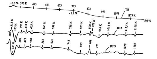
Figure 4. Derivatogramm pattern of the diluvium.
