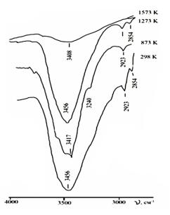
Figure 5. IR absorption spectra of the deluvium and the products of its heat treatment in the region of 4,000-2,500 cm-1.
