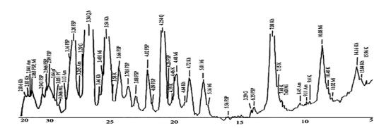
Figure 2. Diffraction pattern of the deluvium. Legends: Kh – chlorites; Fsp – feldspars; Q – Quartz; K- clay minerals; G – Goethite; Mi – micas; Am – amphiboles; Pf – Pyrophyllite.
