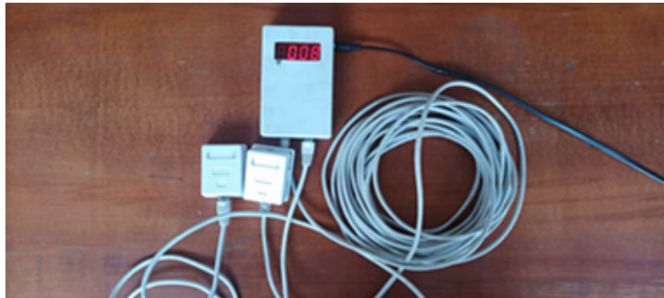
Fig. 3. realized and working Photo of a laboratory sample of the measurement system with sensor blocks and communication cables
