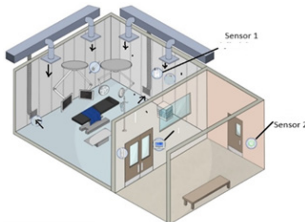
Fig. 1. Locations of components of the pressure difference measuring system located in medical rooms
