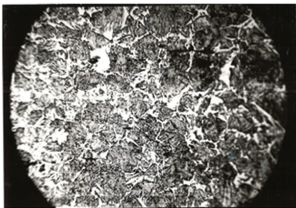
Figure 1. The microstructure of metal into the depth from the cut surface when air-plasma cutting
